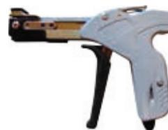
A metal tool which allows to adjust the tightening strength with the screw under the handle. When the set tension is reached, the blade cuts off the tail of the ties without effort and flashes. Suitable for cable ties with width up to 7,9 mm.
